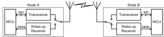
**Figure 1: Example of asynchronous rendezvous using wake-up receiver-enabled wireless sensor platforms.**
