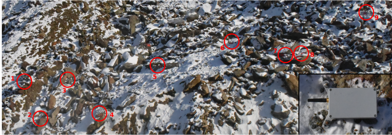
Figure 4.16: Distributed sensor nodes detect trigger events when seismic signals emanating from friction within the rock and sediment mass moving downslope exceed predefined threshold levels. Sensors are located across an area of 50 \times 20 m on a rock glacier with movements of up to 5 m/a [FFBV19]. A close-up of a sensor node shows the mounting at ground level to tightly couple the sensor with the surface.
