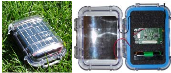
Fig. 1.2: A solar energy harvesting WSN mote packaged in a weather proof case [RKH + 05].
