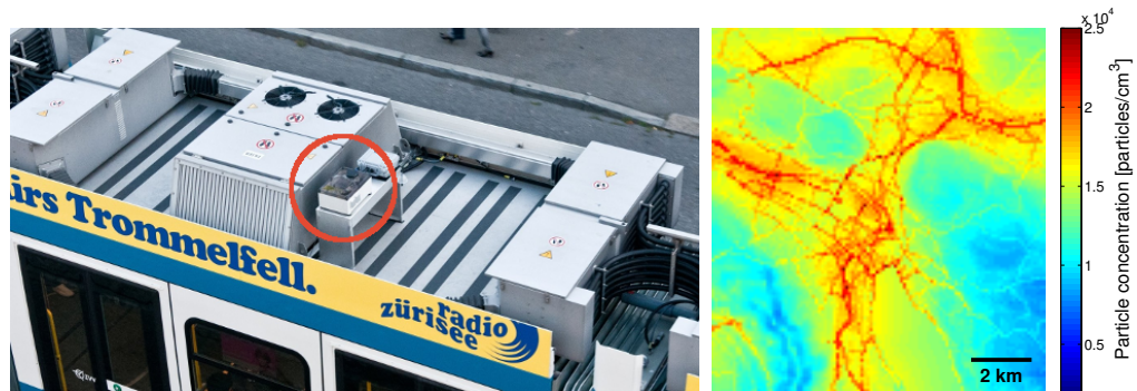
(a) Sensor node on top of a public transport vehicle. (b) Fine-grained pollution map.
