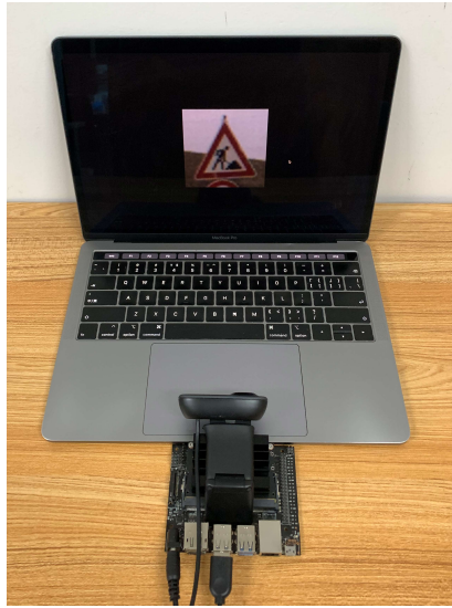
Figure 2.6 Hardware setup to measure the execution time of the nine inference tasks (the photo was for the traffic sign recognition task, i.e. , the GTSRB dataset [59]) on the Jetson Nano embedded platform.
