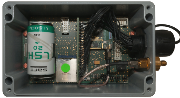
Fig. 1.2 Tinynode 184 sensor node on top of a second-generation Sensor Interface Board (SIB). The 1 GB large SD memory card can store approximately 27 million data packets and is thus well-suited both as a buffer for unsent packets and as a long-term backup medium.
