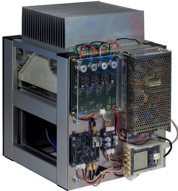
Figure 3.4: The fully integrated solar testbed. The top half represents the mirror-shielded light box with the LEDs mounted below the heat sink. The bottom of the light box consists of a Peltier controlled aluminum plate to maintain a constant temperature of the solar panel during the evaluations (hidden in the shadows). On the right side of the testbed the control circuitry is mounted: the LED dimmer with high dynamic range on top, the SmartLoad (presented in Section 3.4) on the bottom left, and the RocketLogger providing the measurement capabilities and hosting the testbed control (discussed in Section 3.5).
