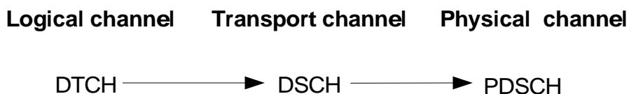
Figure 4-10: Mapping of logical, transport and physical channel in the shared downlink
