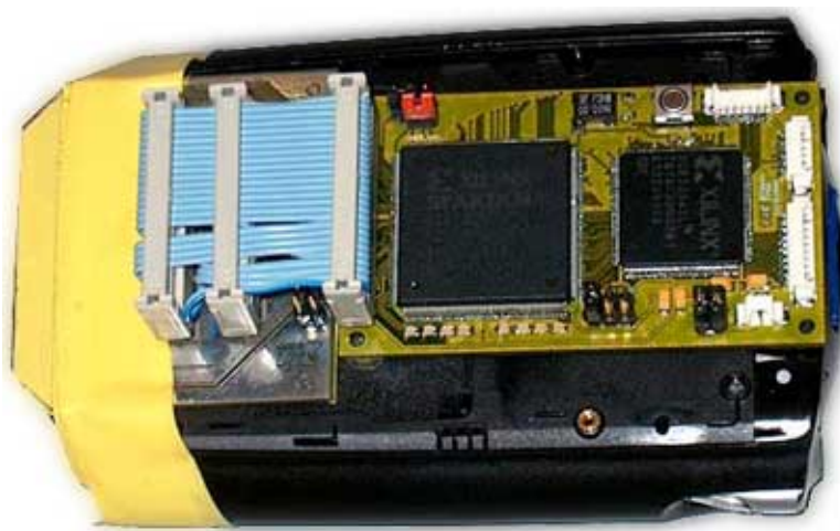
Figure 4-4 BTNODEFPGA - Bridge: Connection to IPAQ The bridge and the cable connects the SRAM interface of the IPAQ expansion port to the IO pins of the BTNODEFPGA board.
