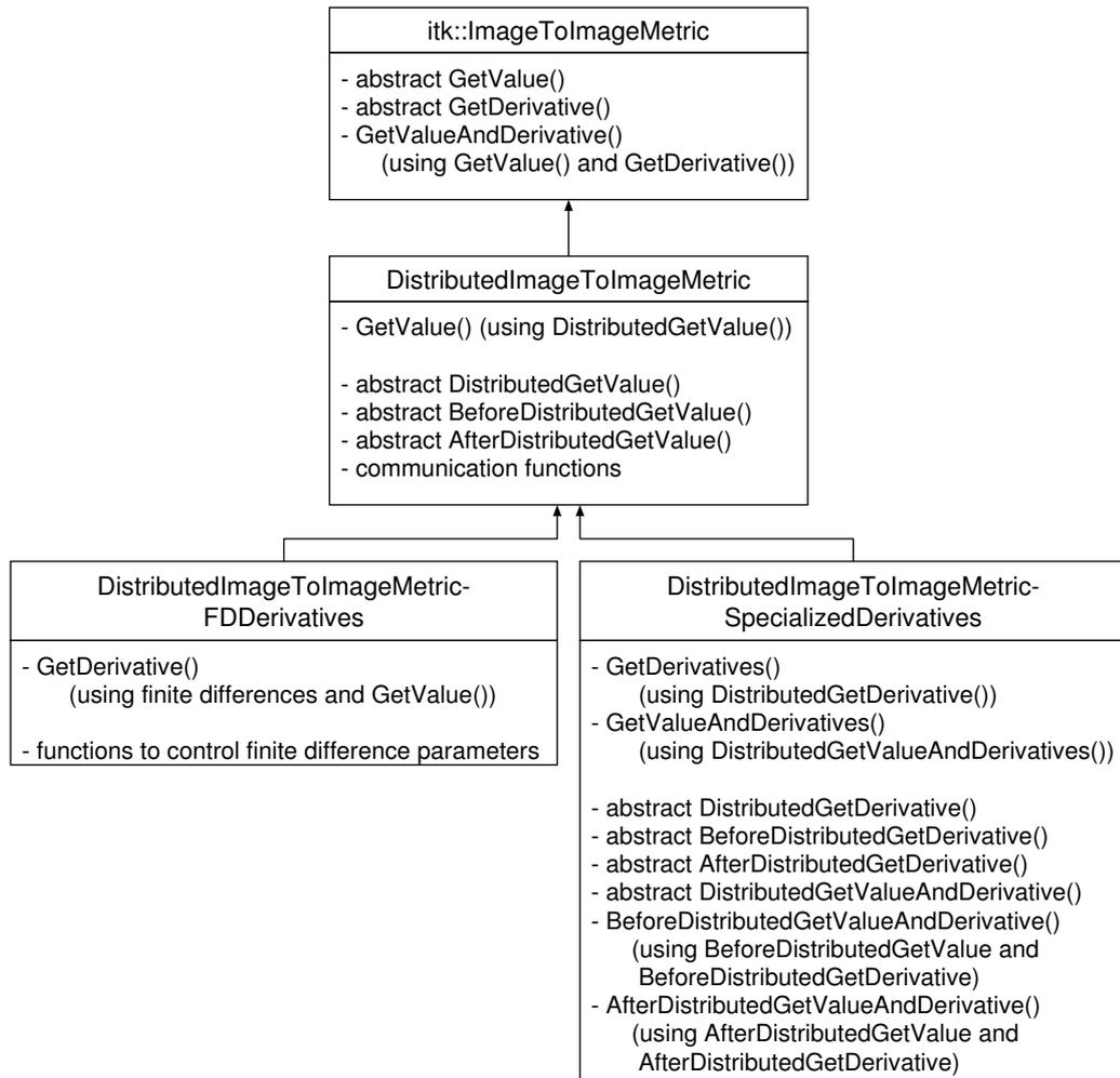
Figure 6.6: Class diagram for the distributed metric modules. New metric functions should either be derived from `DistributedImageToImageMetricFDDerivatives` (for derivative calculation based on finite differences) or from `DistributedImageToImageMetricSpecializedDerivatives` (for derivative calculation by a user defined method).
