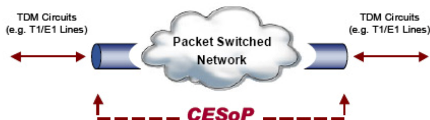
Figure 1.2: Circuit Emulation Services over Packets- A tool to emulate a circuit-switched service on top of a packet-switched network
