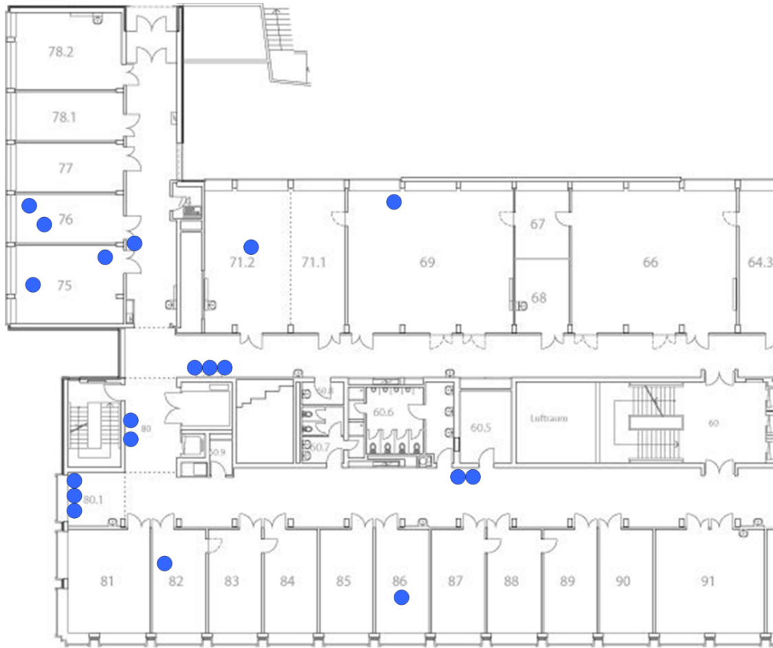
Figure 6-2 Placement of 19 units in an indoor environment. The nodes are powered by USB either directly attached to personal computers or clustered around USB hubs.
