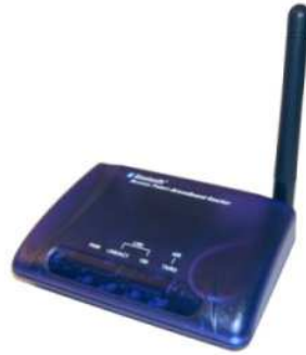
Figure 4.4: The UsbGear USBG-BLUE-RR Bluetooth access point
