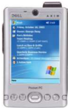
Figure 4.7: Dell's AximX30i PDA can communicate via Bluetooth and WLAN
