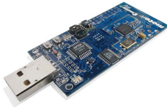
Figure 3-1 Tmote Sky. A next-generation mote platform distributed by Moteiv Corporation.
