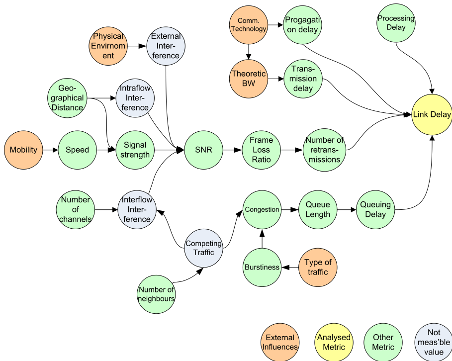
Figure 4.1: Dependencies of the delay metric
