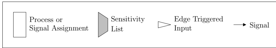
Figure 3.16: Legend for architecture drawings. Whenever a process has an edge-triggered input, it is sequential, otherwise it is combinatorial.
