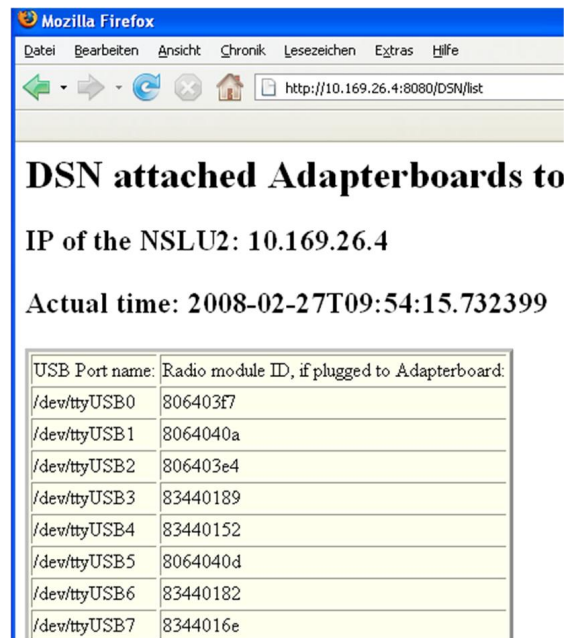
Figure 7.13: The picture shows /DSN/list that informs the user about the DSN configuration. The first time an A80 sends a log message, this page is updated with the new serial port name and the corresponding A80 module ID.
