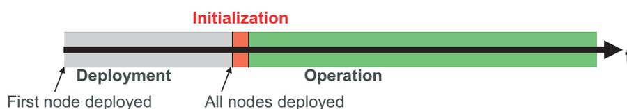
**Deployment** Starts with the first node installed and powered. All the sensor nodes are being deployed at their target location. This phase ends when all nodes are on place - the WSN is fully deployed.
