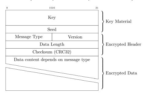
Figure 13: Kraken network packet format.
