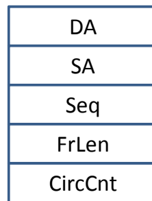
Figure 4.2 The structure of the frame in the simulation
