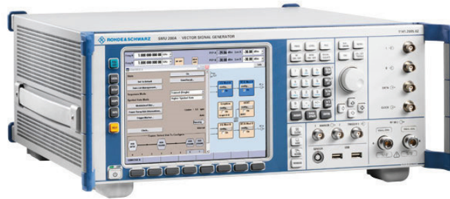
Figure 5.5: R&S Vector Signal Generator SMU200A, used to generate the jamming signals. Source: courtesy of Roschi Rohde & Schwarz AG, Switzerland
