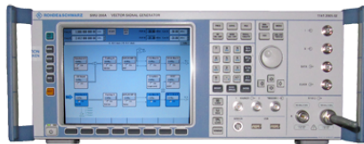
Figure 2.9: The Rhode & Schwarz SMU 200A Vector Signal Generator.
