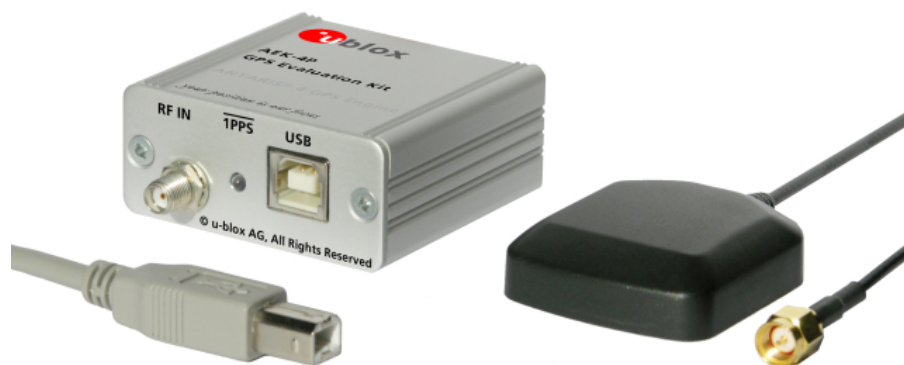
Abbildung 5-1 u-blox AEK 4T Evaluation Kit
