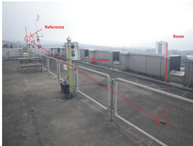
Figure 4-1 The experimental setup on the ETZ rooftop
