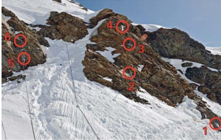
Figure 3.1: AE sensor positions for preliminary experiments at Jungfraujoch
