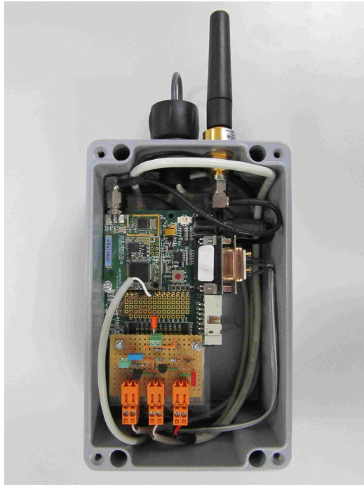
Figure 4-1 Prototype GPS-equipped wireless sensor node (top-view).
