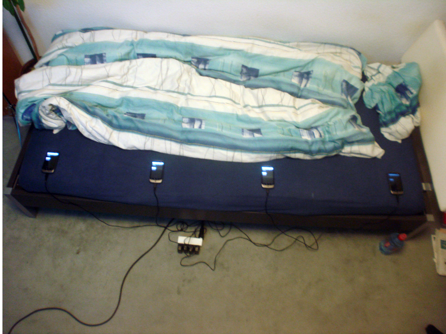
Figure 2.1: Experimental setup of devices in bed to determine the optimal position for recording
