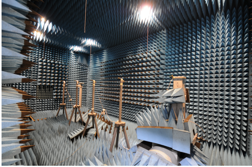
Figure 4.8: Setup of tests in the anechoic chamber. The transmitter node 0 is placed on the stand at the right-hand side of the picture. The four receiver nodes are placed on tripods in a row, on the left-hand-side of the transmitter node.
