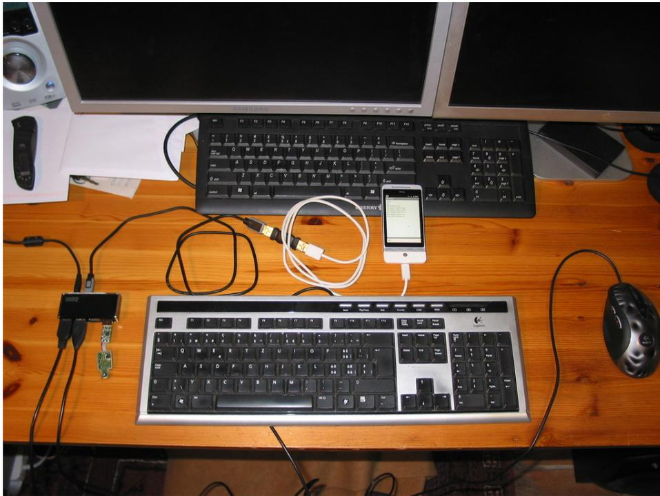
**Figure 2.1:** *The test setup with the self-powered hub. Connected to the phone are a keyboard, a mouse and the ozone sensor.*
