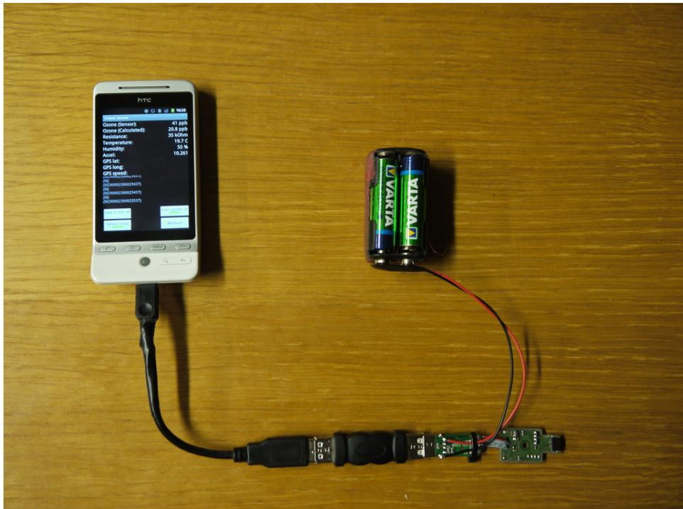
**Figure 2.2:** The final sensor setup, where the sensor is directly connected to the phone. The RS232 $\leftrightarrow$ USB converter and the sensor are powered by the attached battery pack.
