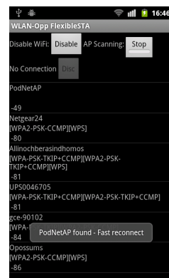
Figure 2.16: Fast reconnection after a connection loss
