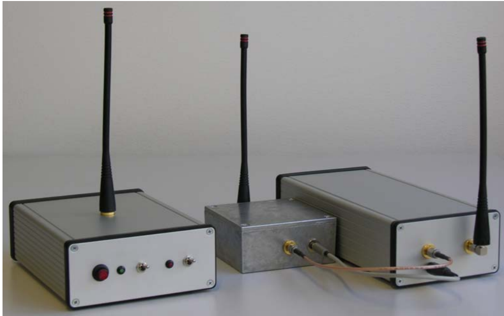
Figure 3.27: Final prototype of the ultra-low power wireless hierarchical sensor network, consisting of (left-to-right) the cluster-head, the OOK demodulator, and cluster node.
