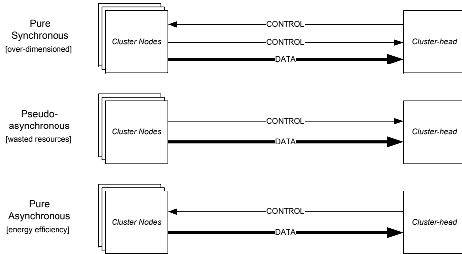
Figure 2.1: Abstract representation of rendezvous schemes for data delivery between a set of cluster nodes and a cluster-head.
