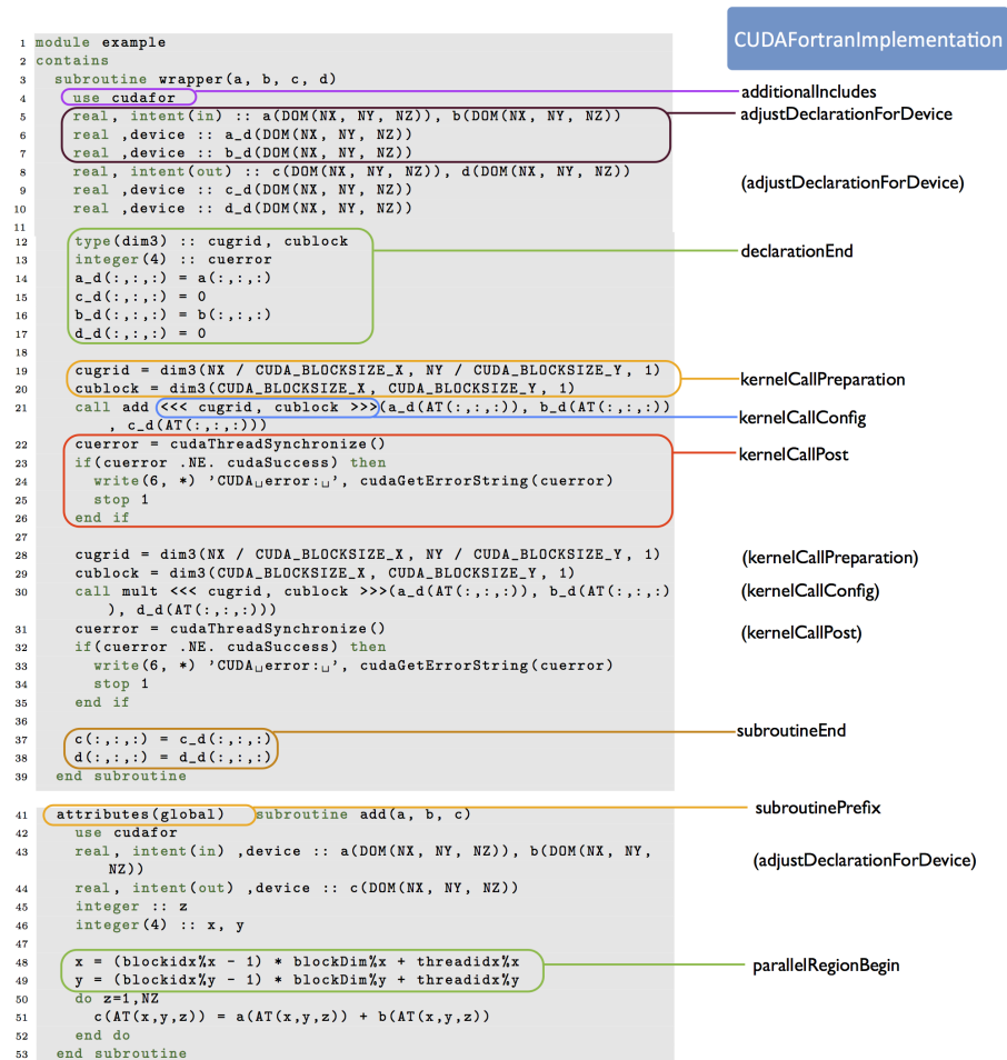
Figure 4.5: Class member functions of “FortranImplementation” classes (Example shown with CUDAFortranImplementation).
