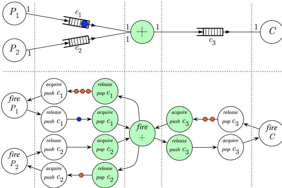
Figure 4.14.: The SDF from the initial example in Figure 4.1 can be modelled as a marked graph. The orange tokens stand for the number of free places in the FIFO. Tokens currently lying on the channel are coloured in blue.
