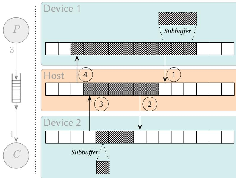
Figure 4.8.: Approach of implementing a channel with triple buffering. Process  $P$  on device 1 sends data to process  $C$  on device 2 using this channel. Tokens are denoted as subbuffers which is a specified region of a buffer of variable size. The complete buffer exists in the memories of both devices and in the host memory. Data transfers (1 and 2) and data invalidation actions (3 and 4) are coordinated by the host memory and are executed on the level of subbuffers.
