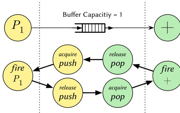
Figure 4.6.: Dependencies between process invocation and channel interfaces. The nodes represent functions calls. For this simple network with two processes and one channel with capacity of one token, the call order has to be a counterclockwise circle, as illustrated.
