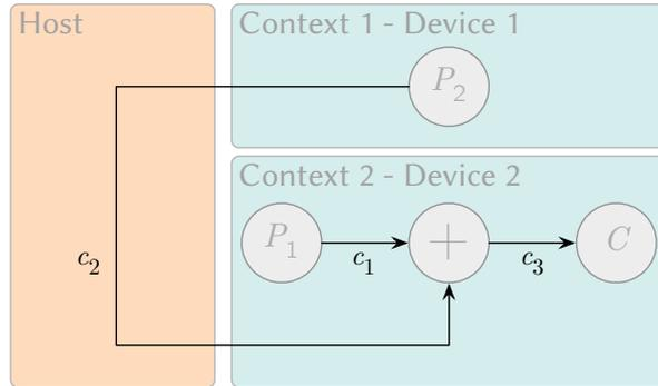
Figure 4.11.: Selection of the correct channel implementation based on the mapping of the processes that are interconnected through it.
