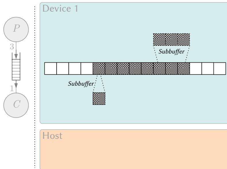
Figure 4.10.: Approach of implementing a channel with single buffering. The process  $P$  sends data to  $C$  using this channel. Both processes are mapped onto the same device. Tokens are denoted as subbuffers which is a specified region of a buffer of a variable size.
