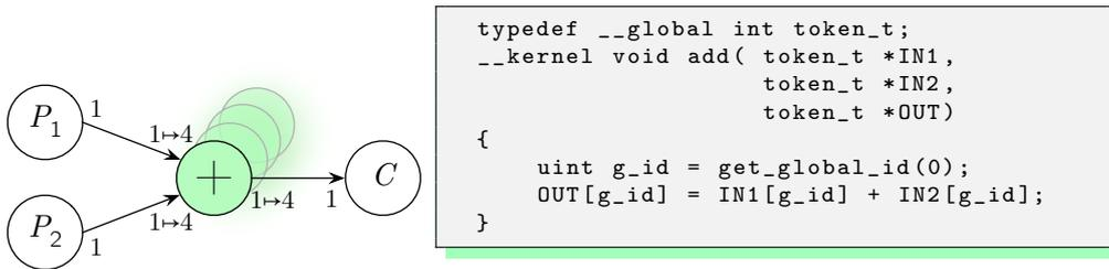
Figure 4.3.: Approach of achieving data-parallelism in an SDF by using four shadow copies. The right hand side depicts the corresponding OpenCL kernel for the (+) process. The token rate of the channels is adjusted accordingly.
