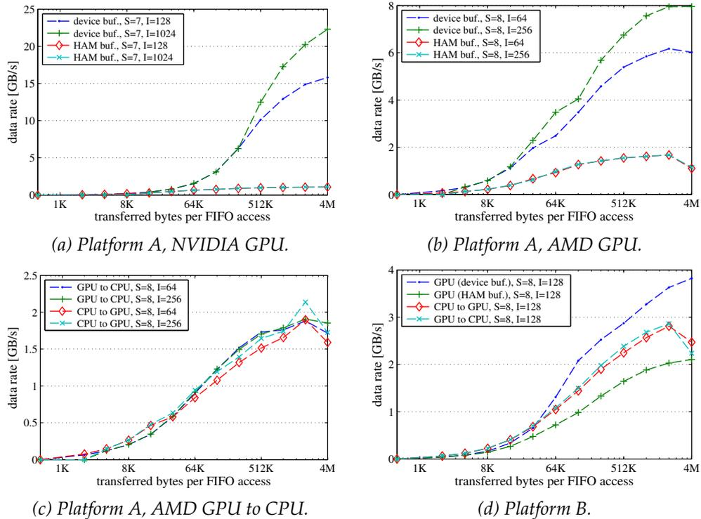
Figure 6.2.: Data transfer rate for different process mappings and channel implementations.
