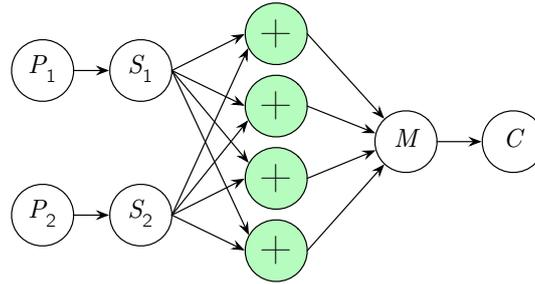
Figure 4.2.: Approach of achieving data-parallelism in an SDF by using splitters ( $S_1$  and  $S_2$ ) and a merger ( $M$ ).
