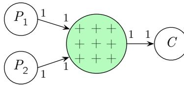
Figure 4.4.: Approach of achieving data-parallelism in an SDF by using inherently parallel operations within a process (in this case a vector addition).
