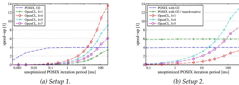
Figure 6.6.: Speedup of the OpenCL and the optimised POSIX implementations versus the unoptimised POSIX implementation.  $I$  denotes the level of intra-process parallelism.
