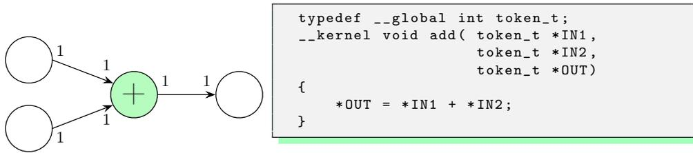
Figure 4.1.: Representation of the SDF process (+) on the left hand side as a functionally equivalent OpenCL kernel.
