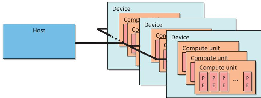
Figure 3.3.: OpenCL system, taken from [1].
