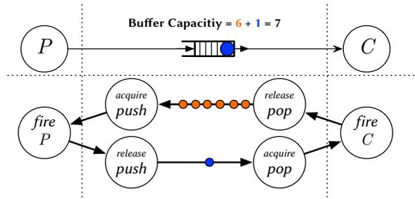
Figure 4.13.: A simple producer-consumer SDF can be modelled as a marked graph that describes the interface dependencies between two interconnected processes through its channels. The orange marks correspond to the free places in the channel, whereas the blue token corresponds to a mark currently lying on the channel.
