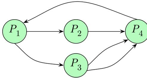
Figure 3.2.: A process network consisting of four processes denoted as a directed graph. The nodes represent the processes, and the arcs the interconnecting channels.
