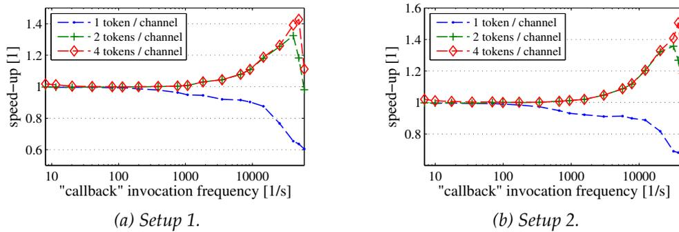
Figure 6.4.: Speed-up of the application in Fig. 6.3 when using the task queue mechanism relative to the execution time when using the direct callback mechanism. The  $x$ -axis denotes the invocation frequency when using the direct callback mechanism.
