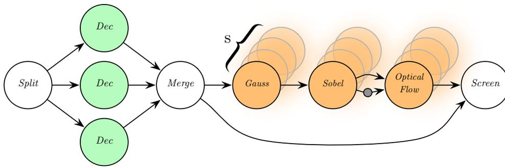
Figure 6.7.: Realistic benchmark application describing an MJPEG decoder and a filter cascade that is applied to raw images.
