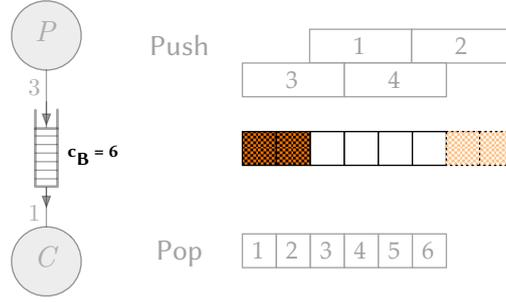
Figure 4.9.: Channel access order for the situation with two initial tokens (dark orange). Push operation 2 will write data over the boundary; this has to be managed by the implementation, which copies the data from this region to the beginning of the buffer after completion.
