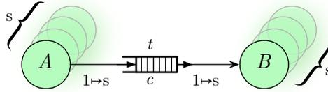
Figure 6.1.: A producer-consumer model for measuring the reachable throughput with parameterised shadow copies  $s$ , token size  $t$ , and channel capacity  $c$ .
