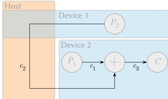
Figure 4.12.: Device 1 has host unified memory. The channel implementation can use this information to select a more performant variant of its channel implementations.
