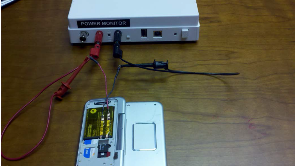
Figure 4.8: Power Monitor setup.
