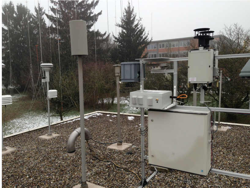
Fig. 4.1.: In the middle of the picture is the OpenSense test box above the white power box. In the background are various NABEL sensor air inlets, which suck ambient air into the measurement station.
