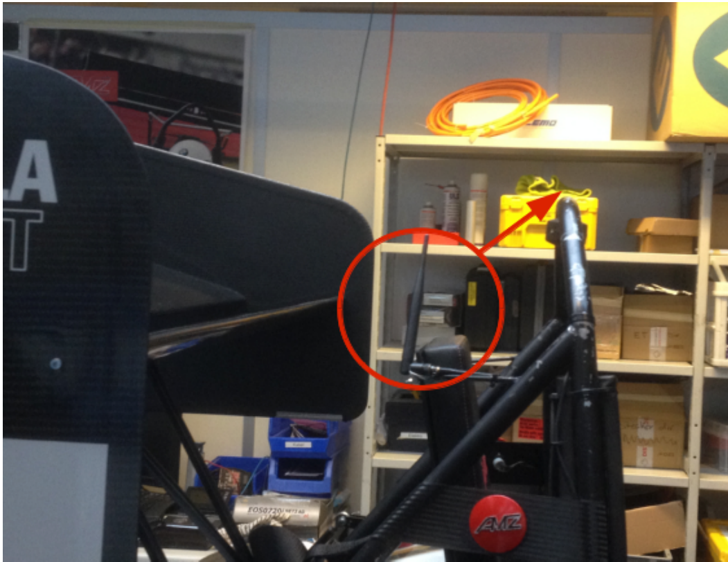
Figure 3.4: Changed positioning of the antenna on the MRH.
