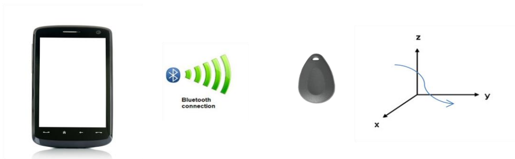
Fig. 1.0: Concept of the project: The sensors measure the movement of the key chain and the data is sent to the mobile phone over a Bluetooth connection.
