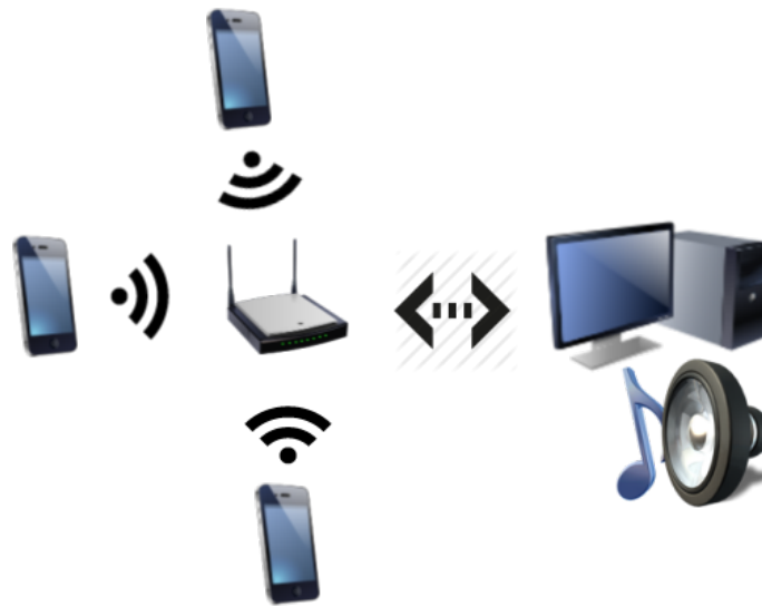
Figure 5.1: Visualization of the application's architecture. The server could also be connected to the network via WiFi, as long as all devices are within the same network.
