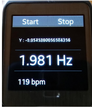
Figure 3.7: The screen of the smartwatch while running the application. The middle line shows the resulting frequency of the FFT.
