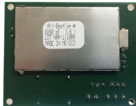
Figure 6-1 Printed circuit board containing the DC-DC converter and the storage capacitors.
