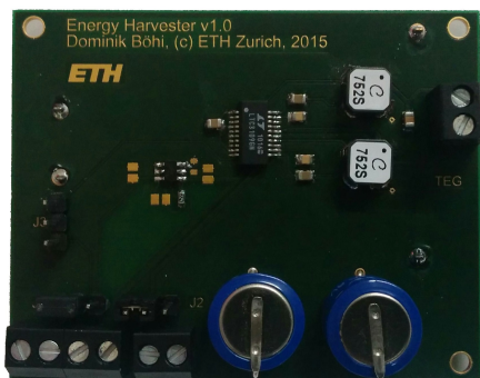
Figure 6-1 Printed circuit board containing the DC-DC converter and the storage capacitors.
