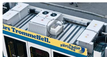
(b) Tram with a sensor node on top.
