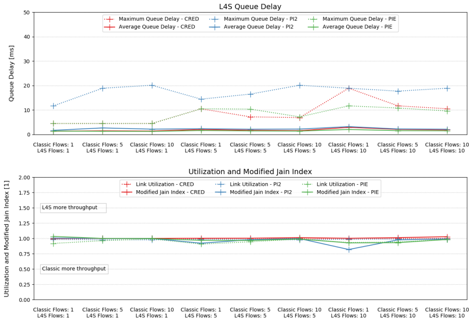
Figure 4.11: Average and maximum queue delays, link utilization and modified Jain index over all flow count combinations for the DualQ Coupled AQM simulations using DCTCP on L4S flows, Cubic on classic flows and activating ECN on the classic flows
