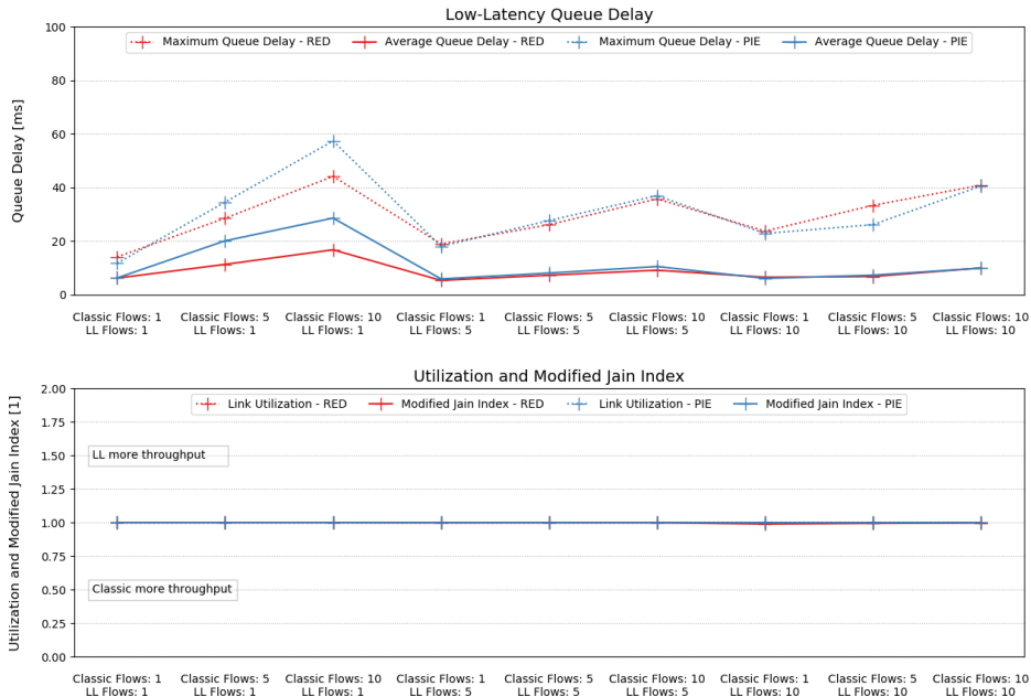
Dual Queue Uncoupled AQM with Scalable Congestion Control on Low-Latency Flows Classic CC: Reno - Scalable CC: DCTCP - ECN on Classic flows: On
