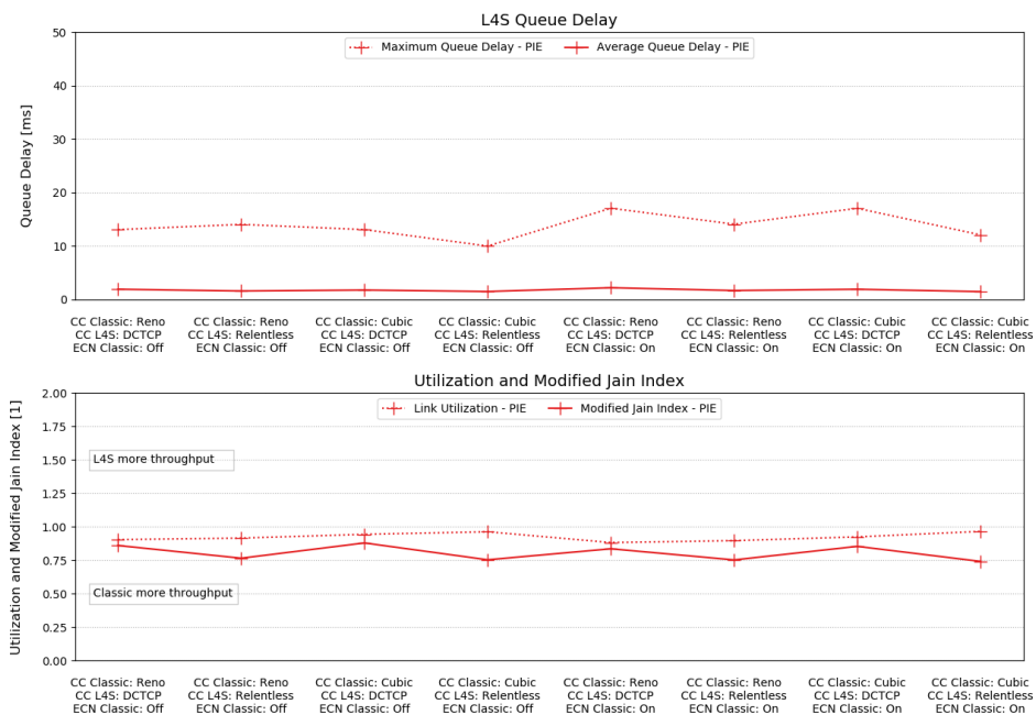
Figure 4.23: Average and maximum queue delays, link utilization and modified Jain index over all available TCP settings for the DualQ Coupled AQM simulations with 5 low-latency and 5 classic flows
