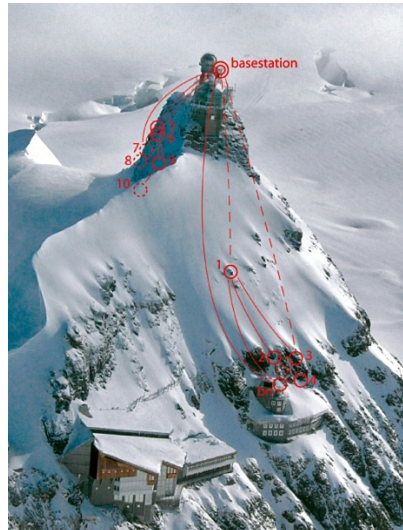
(a) Locations of the sensor nodes. Circles indicate sensor nodes, lines show the network links between them.
