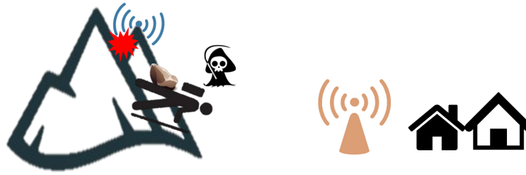
Figure 1.1: In the current system, the event classification only runs on the server. Since the transmission takes some time, there exists certain delay for mountaineers to receive an alarm from the warning system and this delay may cause some damages.
