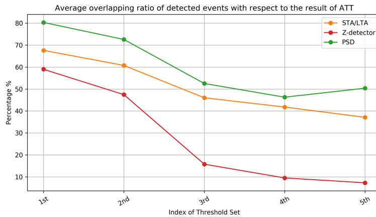
Figure 4.13: The overlapping ratios of detected events with respect to the result of ATT with different thresholds
