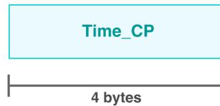
Figure 4.4: The *SCHEDULE REQUEST* packet is a feature of the outsourced scheduler and exclusively contains debug information. Its *arrival* however is important, as it triggers a reply in the form of a schedule which is sent to the CP to be distributed throughout the network.
