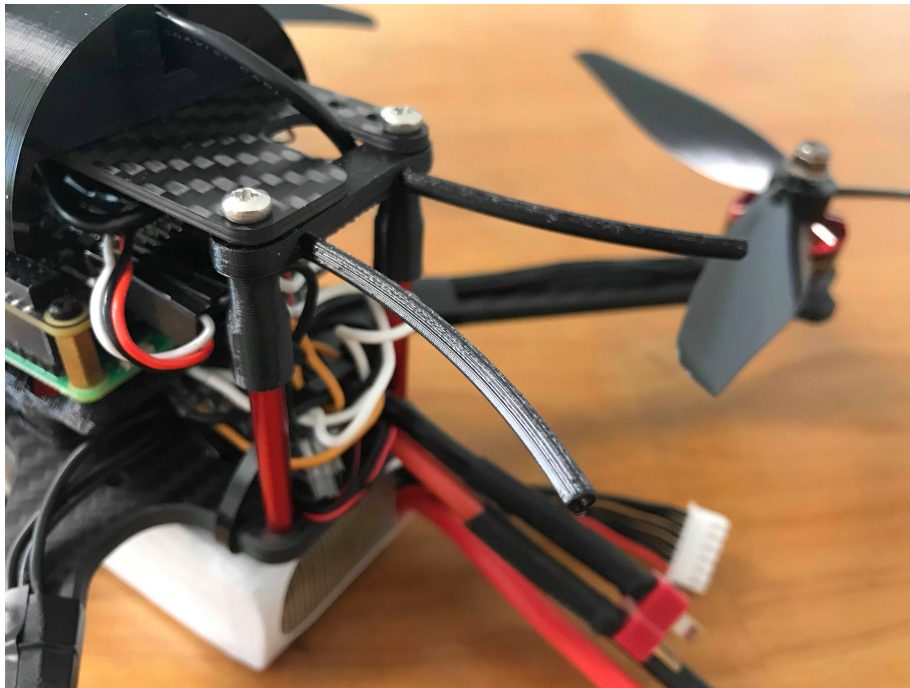
Figure 2.7: A mount for RC receiver antennas makes sure they are kept away from the propellers.
