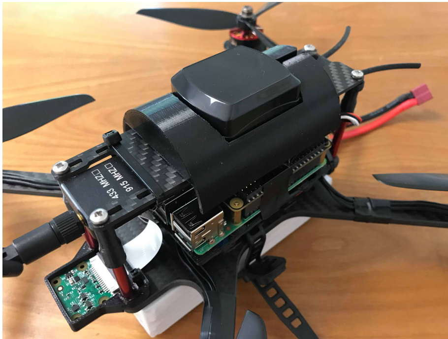
Figure 2.8: The GPS antenna mount helps to keep the GPS antenna safe on the drone. For further use an extension is recommended.
