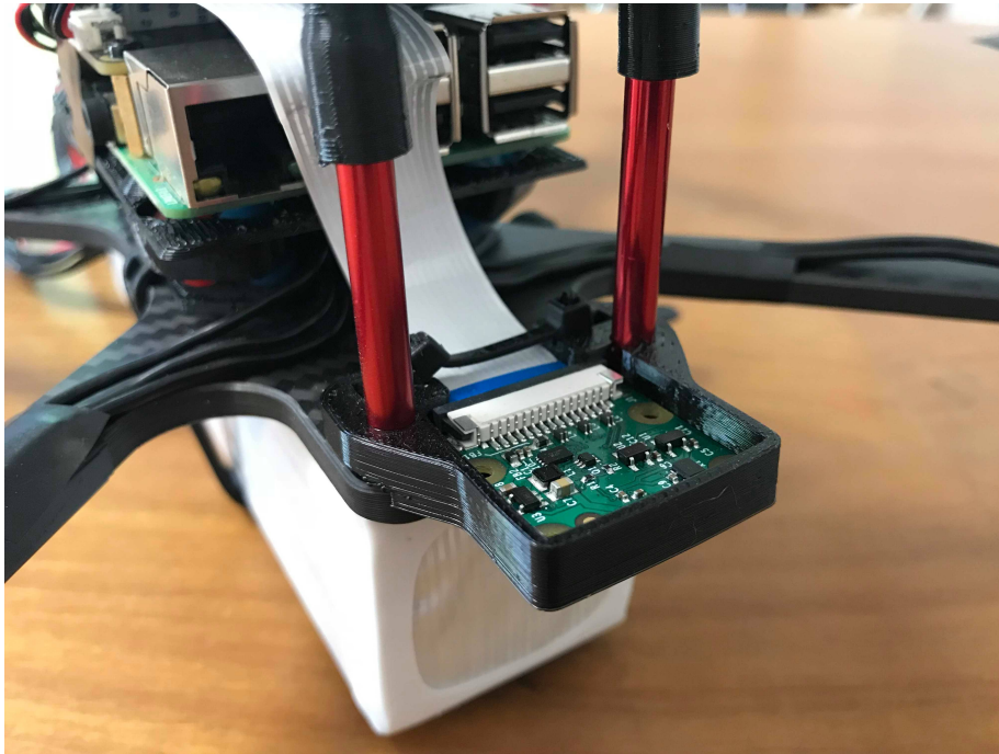
Figure 2.6: Raspberry Pi camera mount holds the camera in front of the frame.
