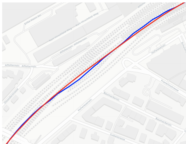
Figure 3.2: Example of a route section, where small deviation of the points leads to unnecessary curvature. The blue line shows the unprocessed route and the red line illustrates the route after discarding points.
