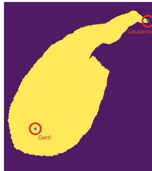
Figure 4.2: Search space of the pathfinding from Geneva to Lausanne. The expanded nodes are shown in yellow and the locations of Geneva and Lausanne are circled in red.
