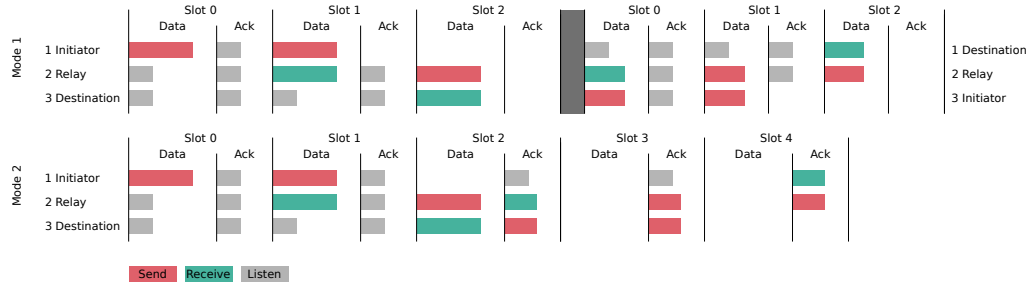
Figure 3.8: Ack mode comparison example 2.
