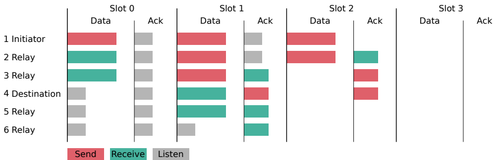
Figure 3.3: Flood with ack mode 1, 3 retransmissions and the maximum number of acks set to 2. All nodes are finished with the flood after slot 2.
