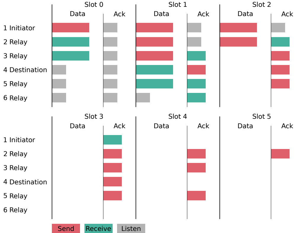
Figure 3.4: Flood with ack mode 2, 3 retransmissions and the maximum number of acks set to 3. All nodes are finished with the flood at the end of slot 5.
