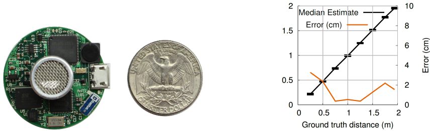
Figure 2.3: Opo only weights 11.4g with a size of 14\text{ cm}^2 (left) and achieves highly accurate ranging results over a distance of up to 3 m (right) [5].
