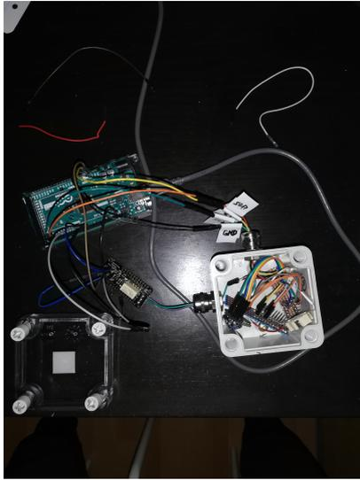
(a) Hydrogen Cell Test Setup
