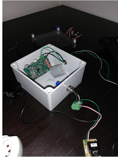
(b) Ionizer Module Test Setup
