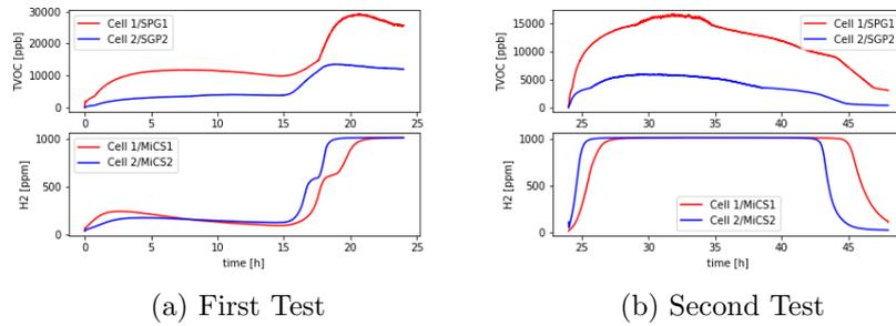
Figure 2.3: pre-calibrated sensor signals of SGP30 (Top), MiCS (bottom)
