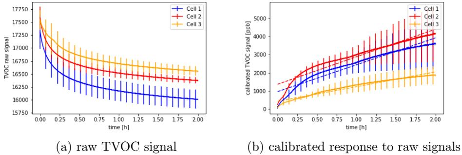
Figure 3.2: Combined results from 30 experiments with hydrogen cells
